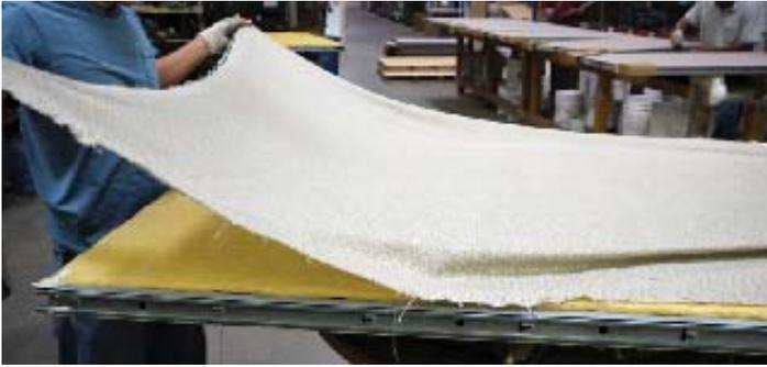
Lay out the new fabric with the correct side up and proper direction (compare with existing panels if unsure). Smooth out any wrinkles that may exist.
