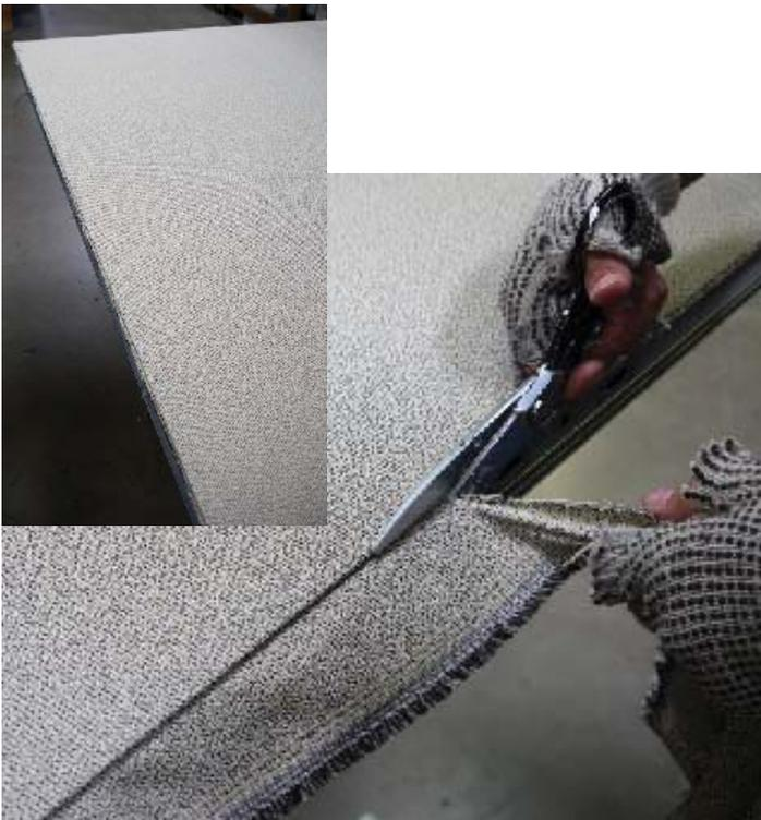
Use the scissors along the rail to trim any excess fabric off of the panel.
